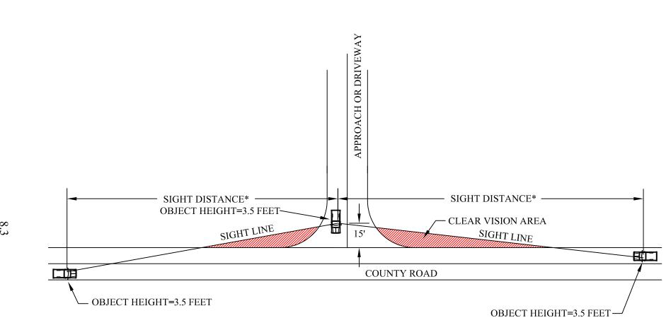
\*SIGHT DISTANCE IS BASED ON THE SPEED LIMIT. SEE SECTION 6.3.4 IN THE LCRC PROCEDURES AND REGULATIONS FOR DEVELOPING PUBLIC ROADS.
